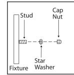
Tuck electrical wires into electrical box and position fixture over studs on mounting bracket assembly. Secure fixture in place with star washer(s) and cap nut(s).
