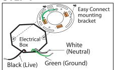
Attach easy connect mounting bracket to electrical box with electrical box screws (not included).
