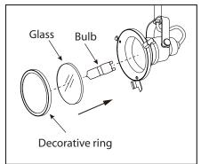
Install specified bulb type and wattage (not included). Position the glass and decorative ring in place.
