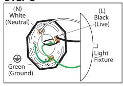
Connect (push) electrical wires from fixture into correct inserts.
